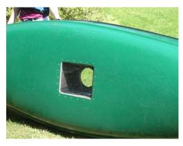
In our canoe we cut a 10" x 13" opening in the center, just forward of the thwart using a saber saw. We obtained a section of Lexan polycarbonate resin thermoplastic intended to replace glass where higher strength is needed. A piece 13"x16" x 1/4" was used to allow 1 1/2" overlap on all four sides. Lexan is a registered trademark of GE, but there are other companies that make similar materials that are as good.
