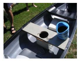
A rectangular box under the shelf is provided to block out most of the light. Our box was made using 1/8" Masonite. If Masonite is used it must be coated with something to keep it from getting wet.
