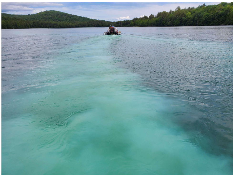
Figure 3: Alum treatment on Long Pond, in Parsonsfield, ME. White aluminum hydroxide ( \text{Al}(\text{OH})_3 ) flocculant can be seen beneath the surface as alum is applied by the barge positioned towards the top of the image.
