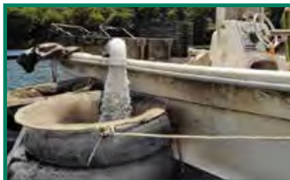
New England Milfoil's Diver Assisted Suction Harvester (DASH). Photo courtesy of New England Milfoil.
